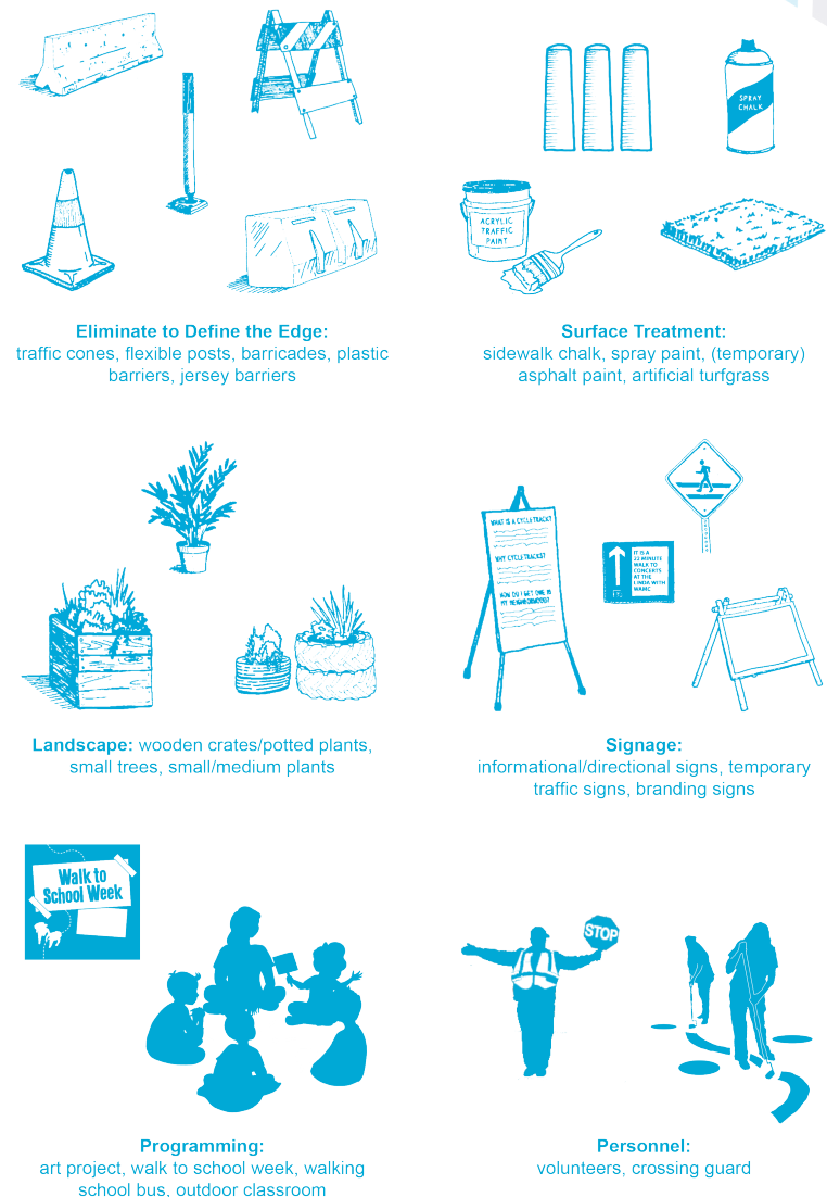
Figure 1: Low cost and removable materials and tactics that are used in Tactical Urbanism. (Source: Jacqueline Sherlock Norheim, Street Plans Collaborative)
