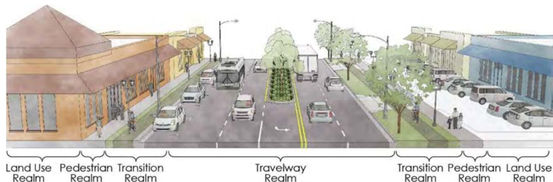
Figure 7-1. Example of cross-section realms from Oregon DOT Blueprint for Urban Design.
