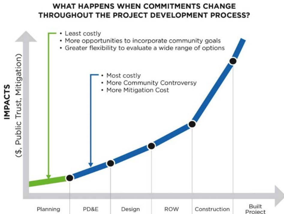
Figure 8-1. Relationship between project phase and cost of design stages.
